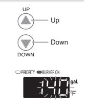
The upper limit of the hot-water supply temperature can be changed to 100°F, 105°F, 110°F, 115°F, 120°F, 125°F, 130°F, 135°F or 140°F.
